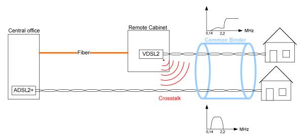
Figure 5: Transmit Spectrum Shaping (TSSi) makes it possible to reduce the transmit spectrum in bands where a Cabinet installation would severely impact the performance of existing DSL installations in same binder.
