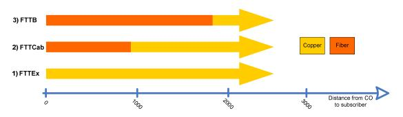
Figure 7: Example: A subscriber living at a distance of 2500 meters from the central office can get a VDSL2 based service based on FTTx scenarios using a mixture of fiber and copper to transport the data.
