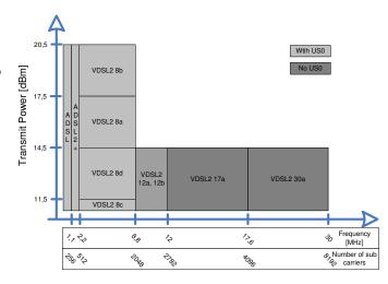
Figure 4: Frequency versus transmit power.
