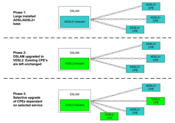
Figure 6: Phase-split deployment of VDSL2 in an ADSL2+ environment.
