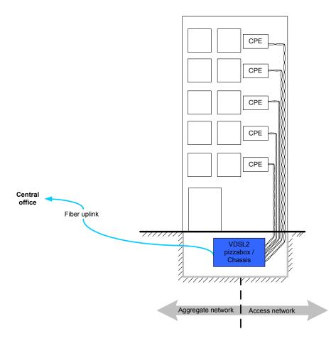
Figure 9: Fiber To The Basement consist typically a fiber connection endpoint in the basement of an apartment building where the existing PSTN wiring is reused for the data connection. Due to the short loop lengths a high bit rate can be offered. This scenario also applies to hotels wishing to provide (wired) internet connectivity to their guests. Both pizzaboxes and chassis types of equipment can be used for this purpose depending on the required port-density.
