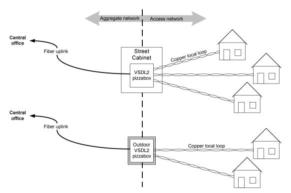
Figure 8: In a Fiber To The Cabinet deployment a fiber is used to connect a remote cabinet to the CO. From the cabinet, the last stretch to the subscribers consists of copper. A VDSL2 pizzabox handles this last-mile connection. ZyXEL also offer outdoor models of the VDSL2 pizzabox that can function in harsh conditions due to the environmentally hardened design.
