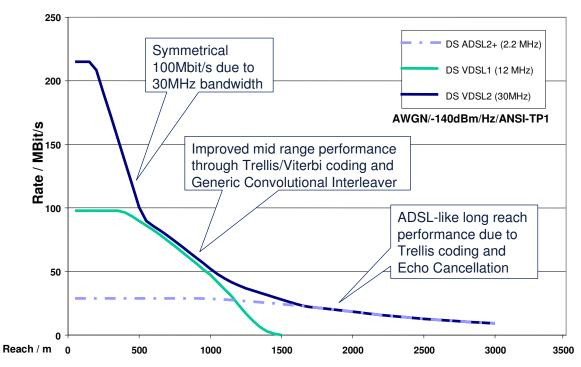
Figure 2: VDSL2 attainable downstream bit rates compared to ADSL2+ and VDSL (Source: DSL Forum)
